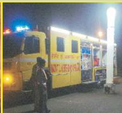
Inflatable light Tower for fire services Inflatable light Tower in a Rescue Vehicle/ Fire Tender
